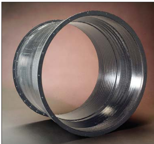
A fan case made from A&P's braided preform, showing the integral flanges and the profile formed on the capstan.
