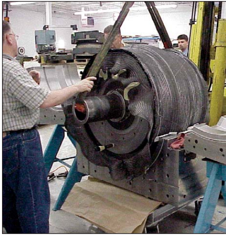
The development resin transfer molding tool, with the braided preform in place on the mandrel, is positioned in the outer mold before it is closed.
