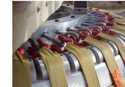
Figure 17. Vectran Belts Connection to Platen
