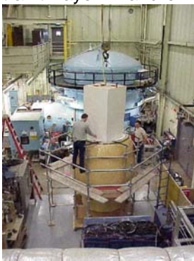
Figure 12. Restraint Layer: Mandrel with Runout Ring
