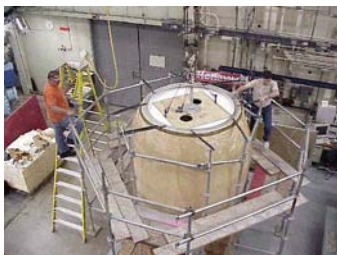
Figure 12. Restraint Layer: Mandrel with Runout Ring
