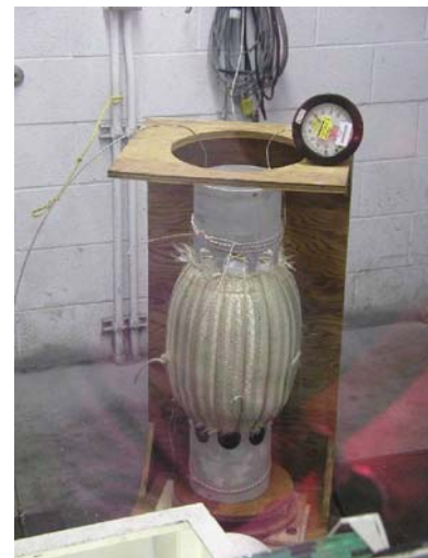
Figure 10. 15% Scale Model – 120-psig Test
