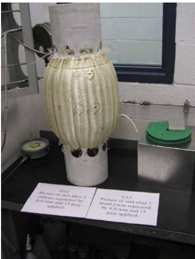
Figure 9. 15% Scale Model During Stability Test
