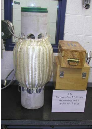
Figure 8. 15% Scale Model During Belt Adjustment
