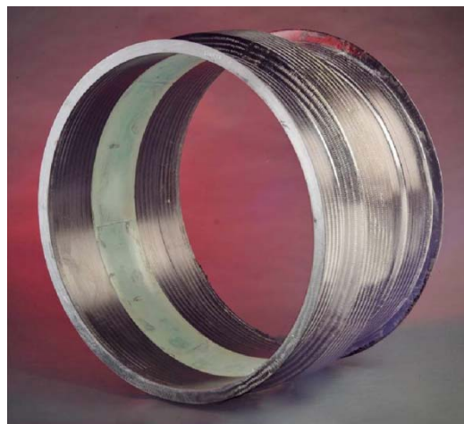
Figure 2.—Composite softwall fan case prototype.
