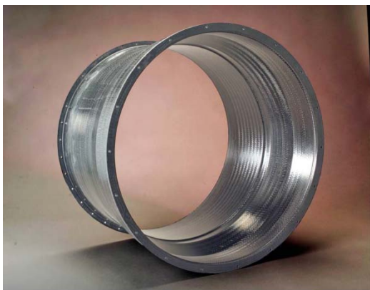
Figure 1.—Composite hardwall fan case prototype.
